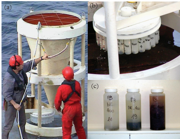
Figure 9.6 Sediment trap. (a) General view (collection surface is 1 \text{ m}^2 ). (b) The carousel with the vials. (c) Vials after sample collection.
