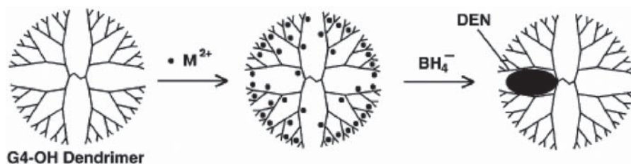
Scheme 11.2 Dendrimer-encapsulated nanoparticle synthesis (Reprinted with permission from reference [112])
