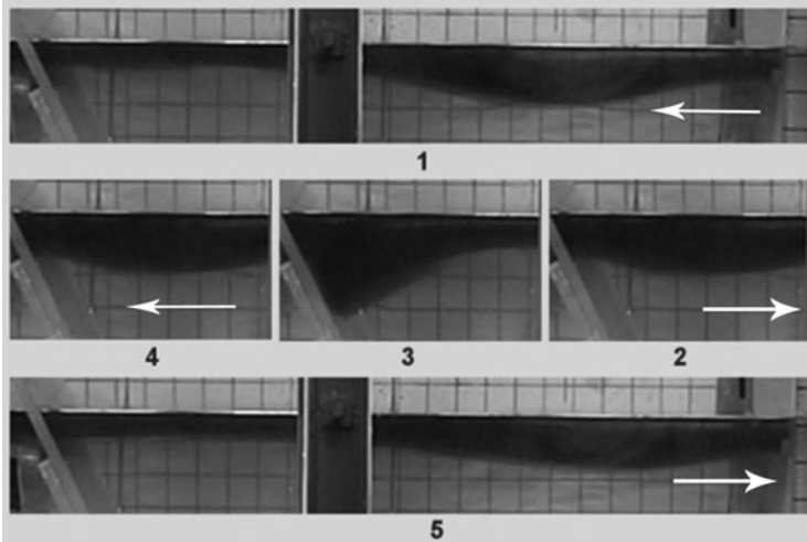
Fig. 4.21 Photographs of wave breaking of the ISW at the steep slope in experiment 2906 (Gorodetska et al. 2012, Chap. 3, this volume)
