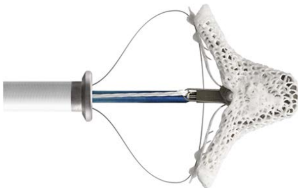
FIG. 32.15 MitraClip device. The MitraClip device is a 4-mm-wide metal (current device is cobalt/chromium) implant with two polyester-covered arms that open to about 2 cm (7–8 mm on either side of a center post). (Courtesy of Abbott, Abbott Park, IL.)
