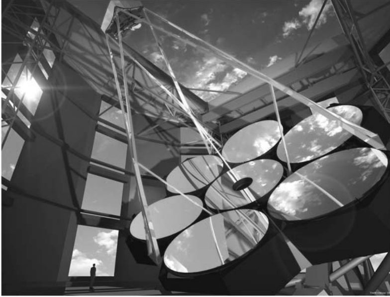
Fig. 11.2. Concept design for the Giant Magellan Telescope, which uses seven 8.4m mirrors on a common mounting (Gunnells et al. 2004). (© Todd Mason/Carnegie Observatories.)
