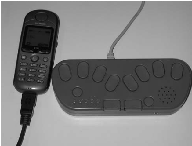
Figure 9: The paddy, an assistive device for users with visual impairments allowing fast and efficient text input.
