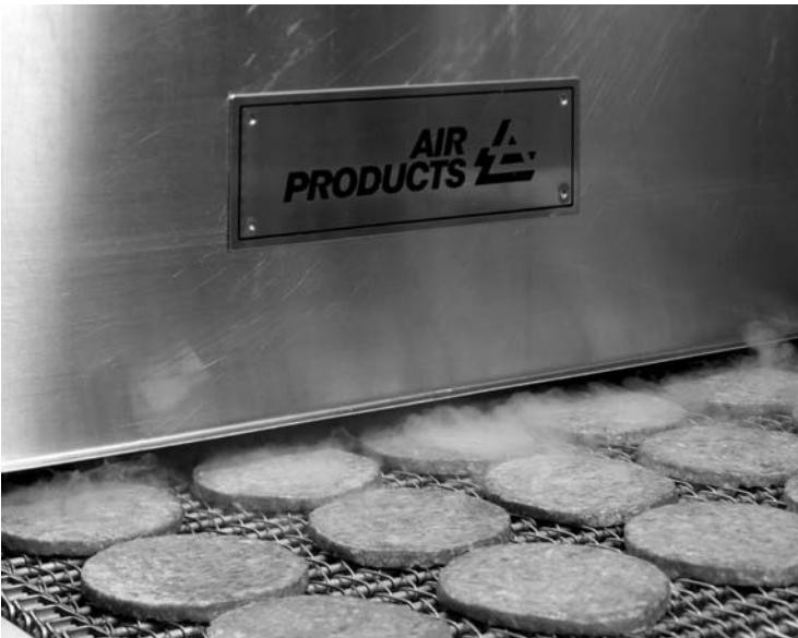
FIGURE 17.4 Examples of cryogenic freezing of foods (Source: 8 1996 Air Products and Chemicals, Inc.; photograph courtesy of Air Products and Chemicals, Inc).
