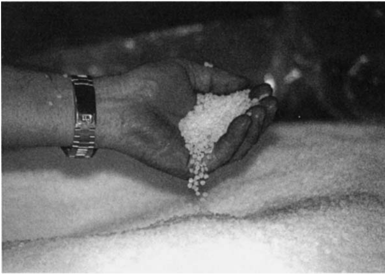
FIGURE 19.2 Polyethylene pellets (Courtesy: Rodeo Plastic Bag and Film, Inc., Mesquite, TX).
