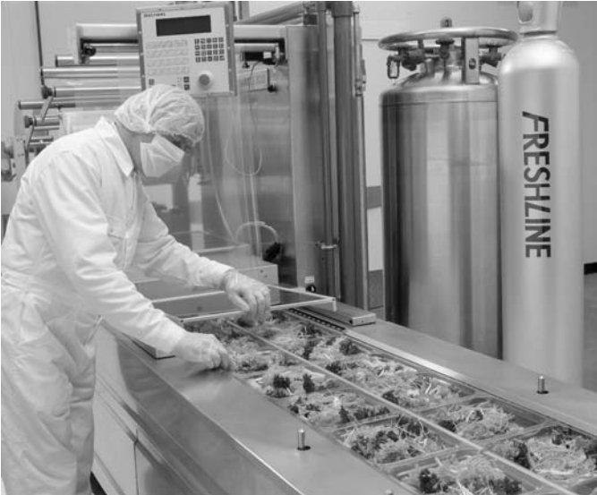
FIGURE 17.3 MAP system for ready to eat salads in a tray. (Source: photograph courtesy of Air Products and Chemicals, Inc).
