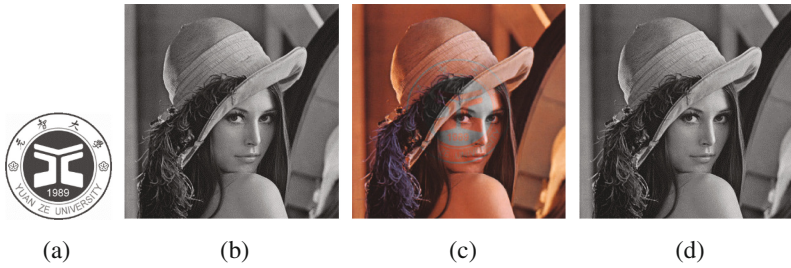
Fig. 5. The experiment of case 1. (a) is the watermark (b) is original image (c) is the watermarked image (d) the hard printed result.
