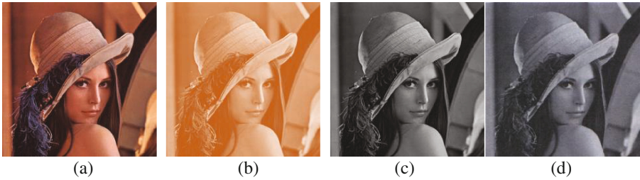
Fig. 3. The test of lemma 1. (a) is the original image (b) is the yellow version image (c) is the gray image which converted from (a) or (b) (d) is the printed and then hard copy image
