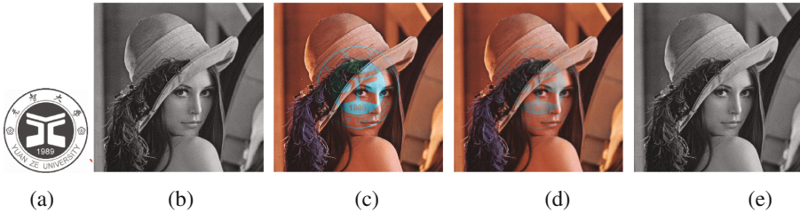
Fig. 8. The experiment of case3 (a) is the watermark (b) is original image (c) is the watermarked image with hue modification (d) is the watermarked image with saturation modification (d) the hard printed result.
