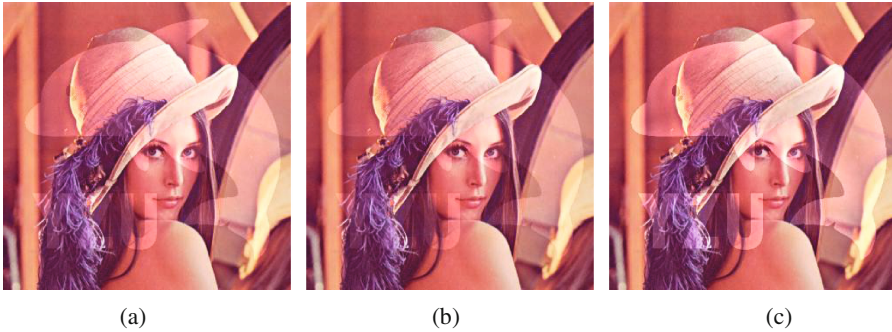
Fig. 3. Comparison of visible watermarks obtained using different stamping schemes: (a) Uniform strength watermarking, (b) HVS watermarking, (c) the proposed method.
