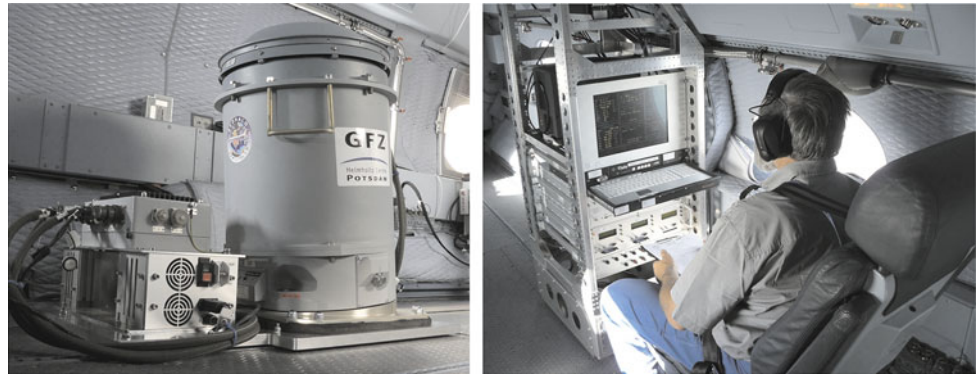
Fig. 1 The equipment mounted inside the HALO aircraft: gravimeter Chekan-AM (left) and the operator rack (right)
