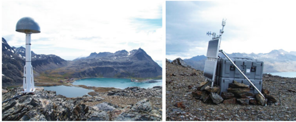
Fig. 2 GNSS antenna and radome on 1-m mast ( left ) and aluminium pipe frame with electronics and auxiliary equipment ( right )
