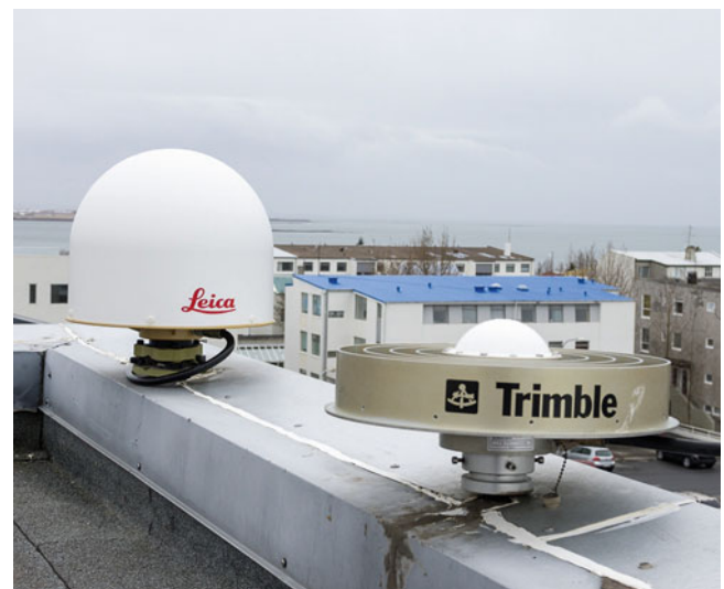
Fig. 5 Temporary Trimble antenna (REY2) installed at the IGS station Reykjavik (REYK, Leica antenna)
