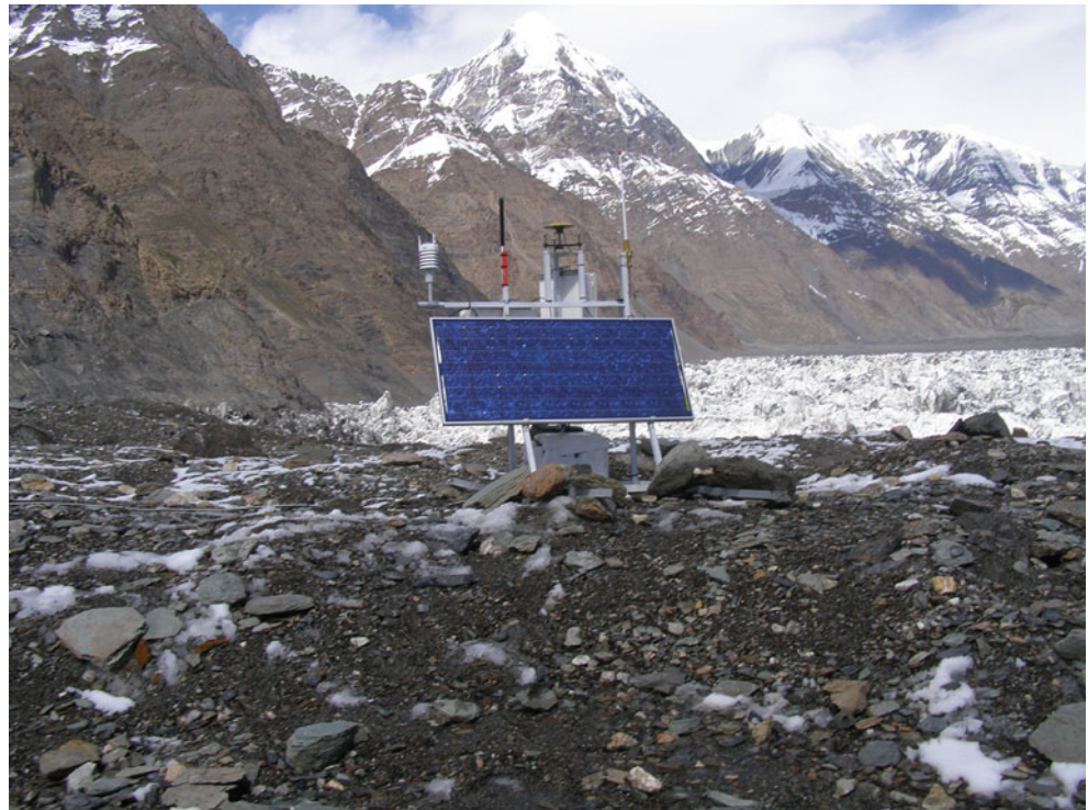
Fig. 3 Kinematic ice dam station (ICED) with a Topcon GNSS receiver, a Vaisala WXT520 weather sensor, power supply and HF radio antennas
