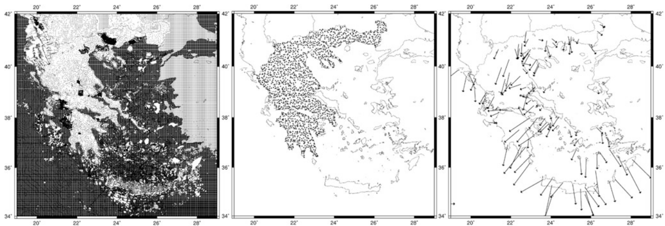
Fig. 1 Distribution of local gravity ( left ), GPS/Levelling ( centre ) and deflections of the vertical ( right ) data in Greece for GOCE GGM validation
