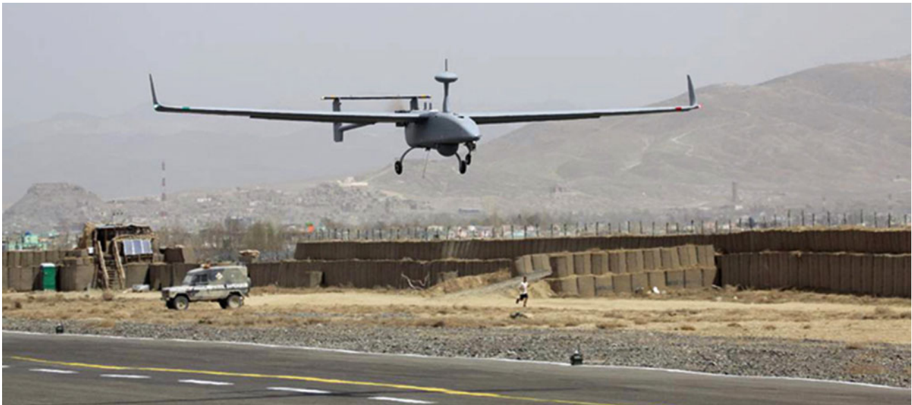
Fig. 5 Photo shows an example of a moderate wingspan UAV that could immediately be used for local and regional ALS data collection
