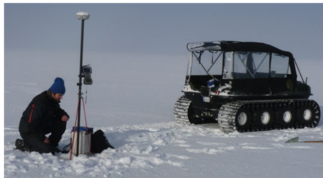
Fig. 2 Gravity surveys and GNSS positioning on Väinameri Basin, a lightweight amphibious crawler was used for transport
