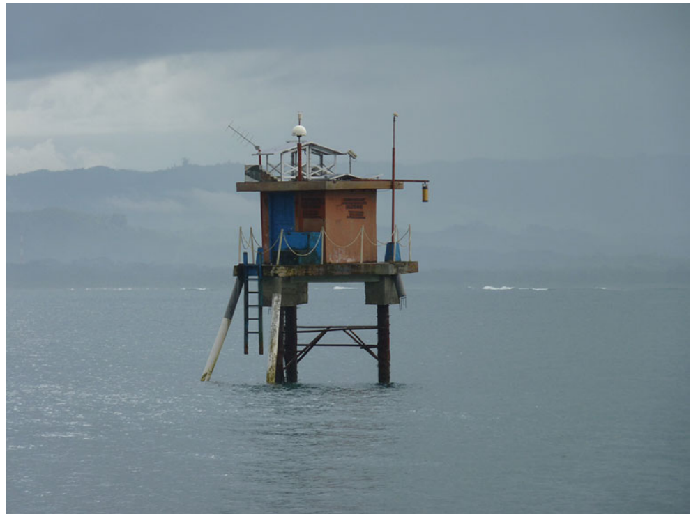
Fig. 2 Tide Gauge at Pangandaran (PANG, Indonesia). The antenna of the GNSS, which monitors the height and vertical motion of the tide gauge, is located on the roof of the tide gauge hut
