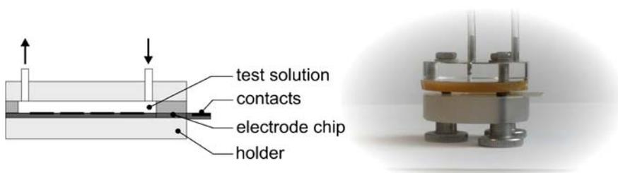
**Fig. 18** Schematic view of the measuring cell used for the impedimetric detection of autoantibodies based on a screen-printed electrode chip
