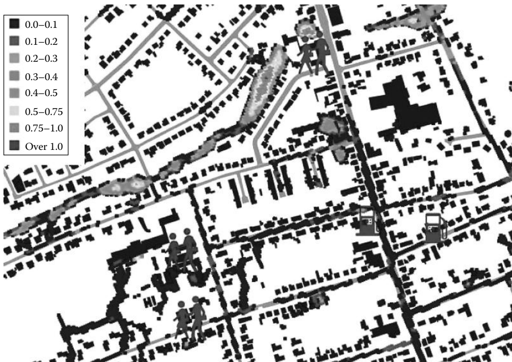
FIGURE 6.6 Example of GIS theme showing specific buildings. Flood levels are pictured together with the location of schools, kindergartens, and gas stations. (From DANVA, Urban Climate Change [Original title: En kagebog for analyser af klimaændringers effekter på oversvømmelser i byer], 2011.)
