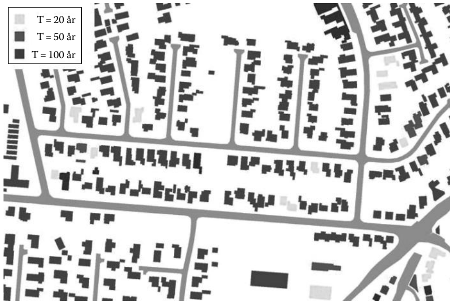
FIGURE 6.3 Example of GIS theme of the houses flooded at different return periods. (From DANVA, Urban Climate Change [Original title: En kagebog for analyser af klimaændringers effekter på oversvømmelser i byer], 2011.)
