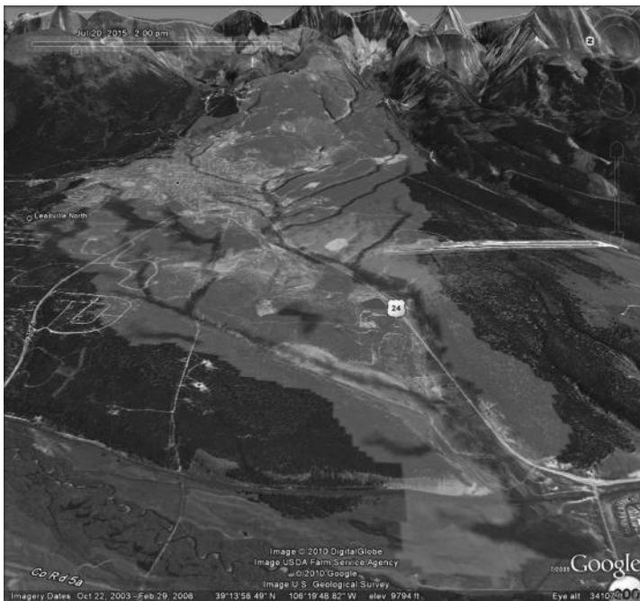
FIGURE 17.3 (continued) Selected frames from a loop showing the depth of water on a land surface using Google Earth 3-D terrain and imagery for a 100-year return period event (1.73 in. in 2 h) at California Gulch. The second frame 17.3b) shows minimal overland flow conditions and channel flooding in the upper part of the watershed 2 hours after cessation of rainfall. The third frame 17.3b) shows that the floodwave propagated to the lower areas of the watershed and caused significant overbank flows.
