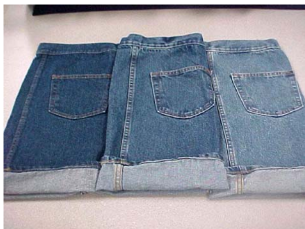
Fig. 7 Enzyme treatments in denim process: ( left ) amylase desized, ( center ) cellulase abrasion, and ( right ) laccase/mediator decolorization
