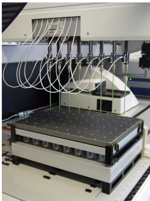
Fig. 3 Photograph of a bioreaction block with 48 stirred-tank reactors on a 10 milliliter-scale at the working-table of a liquid handler
