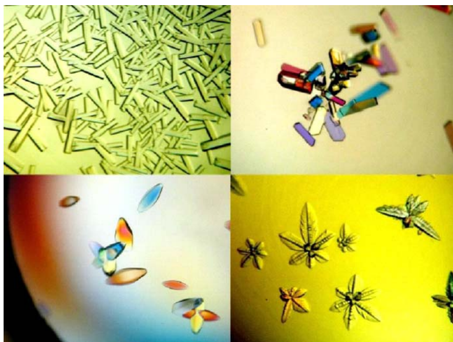
Fig. 10 Different morphologies of crystallized proteins (from [138], with permission from Wiley)
