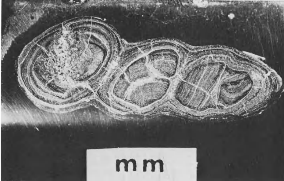
Fig. 19. Polished section of nodule very poor in clay from same box core as nodule in Figure 17 (box core 23, RP8-OC-76). Oblique illumination. The oxides are gray to black, and the thin white seams are clay-filled veinlets and partings between oxide layers. Compare with section shown in Figure 17. This nodule contains very little clay (about 5 percent). The low nickel and copper content shown by the bulk analysis (below) is due to presence of amorphous oxides, not clay, as shown by the Fe content and Fe/Mn ratio.
