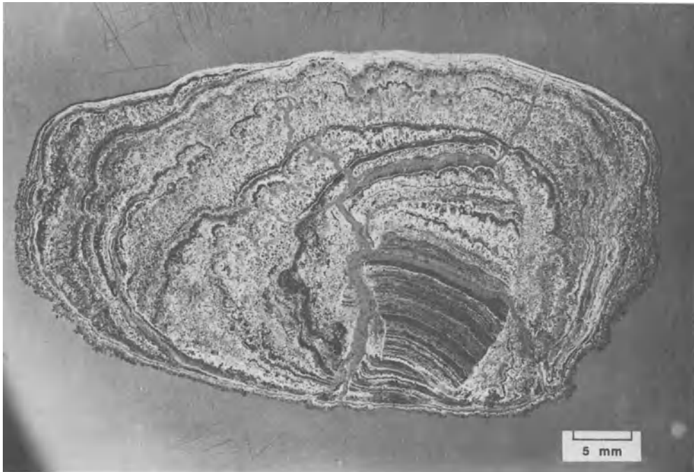
Fig. 11. Polished section of nodule NP 60A-10. In this whole cross-section, viewed in vertical illumination, the internal structure of the nodule is shown in natural orientation. The top and bottom photographs shown in Figures 9 and 10 are of the same nodule. The morphology of the nodule was termed "irregular discoid". Note that the crustal zone over much of the top is clearly more dense and highly reflective than along much of the bottom. The overall growth structure consists of wedging zones of oxides rich in clay around a core which is a piece of an older nodule. The older nodule evidently was much different in internal structure. A complex growth history is suggested.
