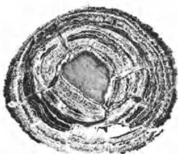
Fig. 3. Internal structure of manganese nodules. Type A: irregular or ellipsoidal nodules with nuclei of fragmented older nodules composed of the \gamma - \text{MnO} phase, and with surrounding 2-5 mm thick layers composed of the \gamma - \text{MnO} and 10\text{\AA} manganite phases. Type B: spherical nodule with continuous concentric thin layers composed of the 10\text{\AA} manganite phase. Scale bar: 1 cm.
