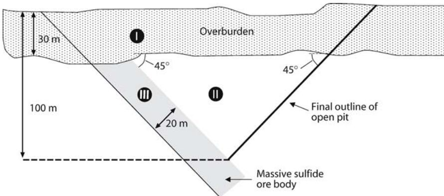
Fig. 9.4. Vertical section to calculate the waste:ore ratio
