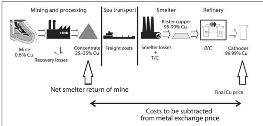
Fig. 7.1. Flow sheet for the recovery process copper
