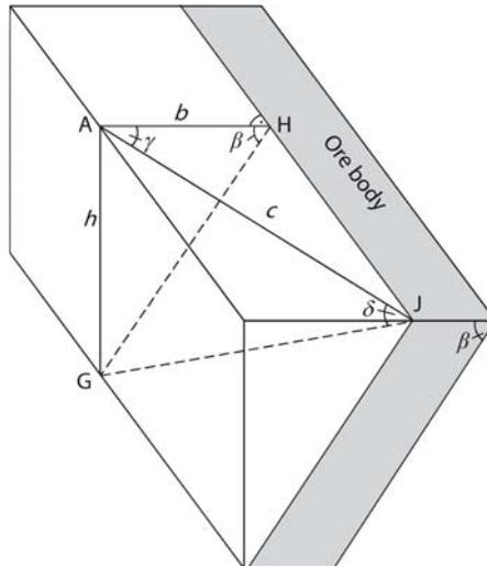
From the profile  $\overline{AC}$  (Fig. 2.2a) the true thickness  $M_w$  can be determined as
