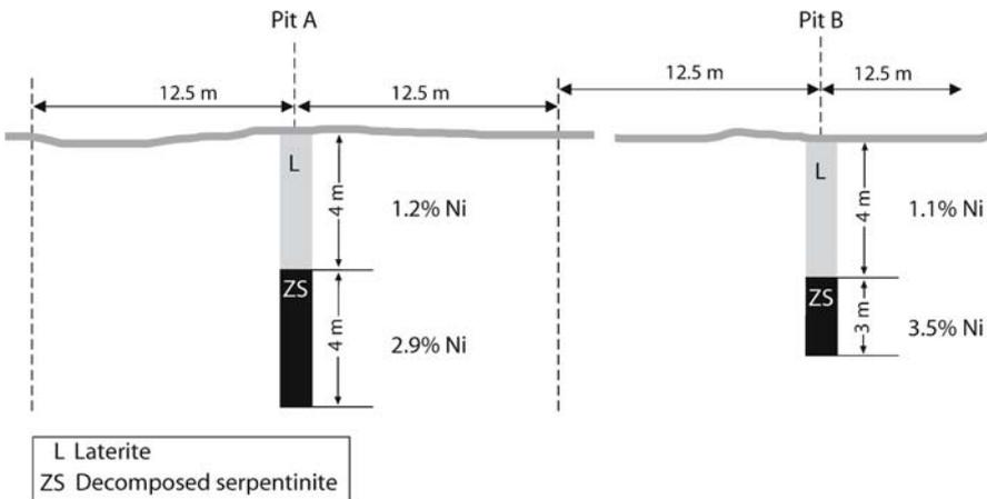
Fig. 2.6. Pit sampling in a nickel laterite deposit
