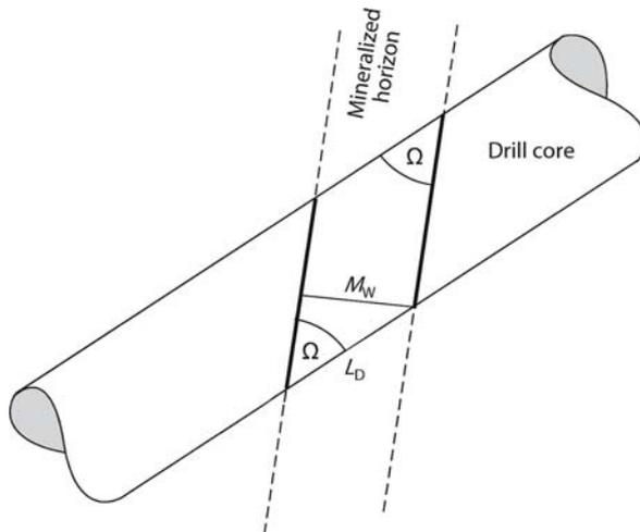
not have to know anything about strike or dip of the ore horizon. With this angle  $\Omega$  and the apparent thickness in the drill hole  $L_D$  we can determine the thickness of the ore horizon  $M_W$ , meaning the normal distance between foot and hanging wall measured at right angles, which is
