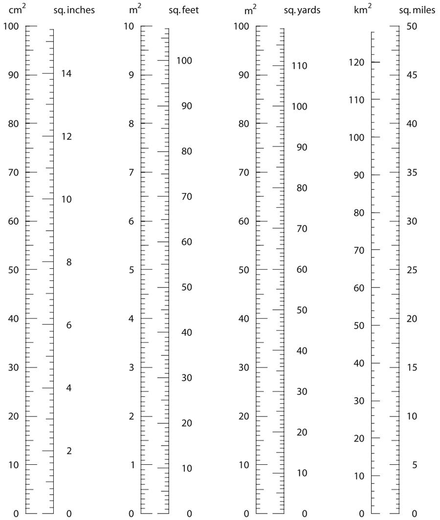
Fig. A2. Conversion between common square measures in the imperial and metric systems
