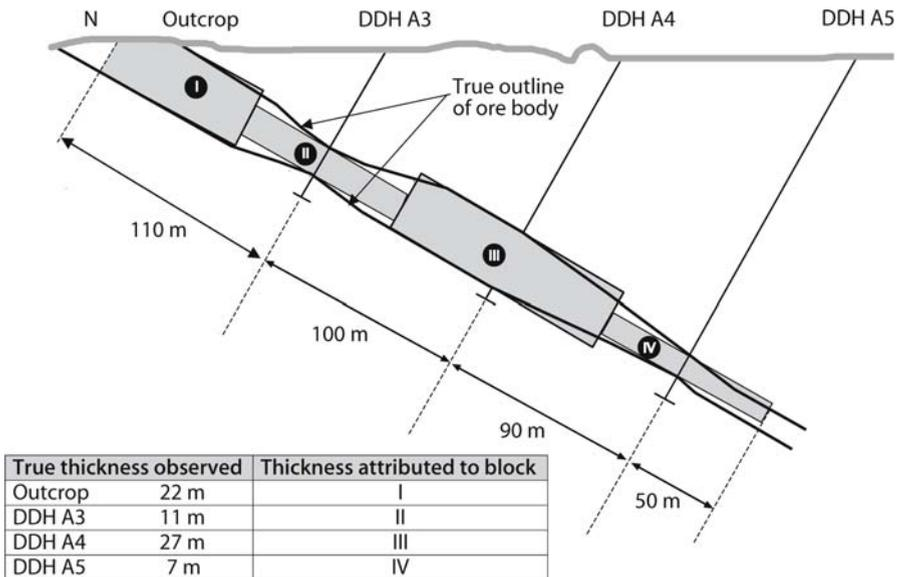
Fig. 2.3. Cross-section for reserve calculations with blocks
