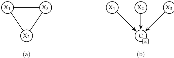
Fig. 7.10. (a) A functional relation f(X_1, X_2, X_3) is to be enforced. (b) A constraint over X_1 , X_2 , and X_3 is enforced by instantiating C to on .
