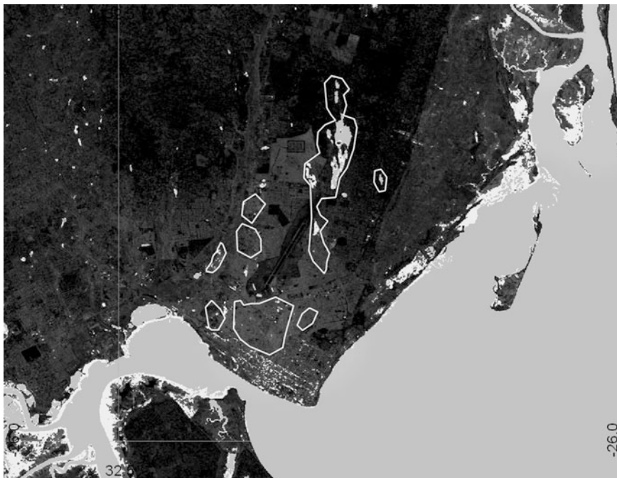
Fig. 11.3 Maputo, 20 May 2000. LANDSAT 7 ETM multispectral satellite image taken 4 months after heavy rainfall, with the areas identified by the USGS (2000) study highlighted. According to the MNDWI, bodies of water are shown in grey and moist soil in white (formulated by Braccio)
