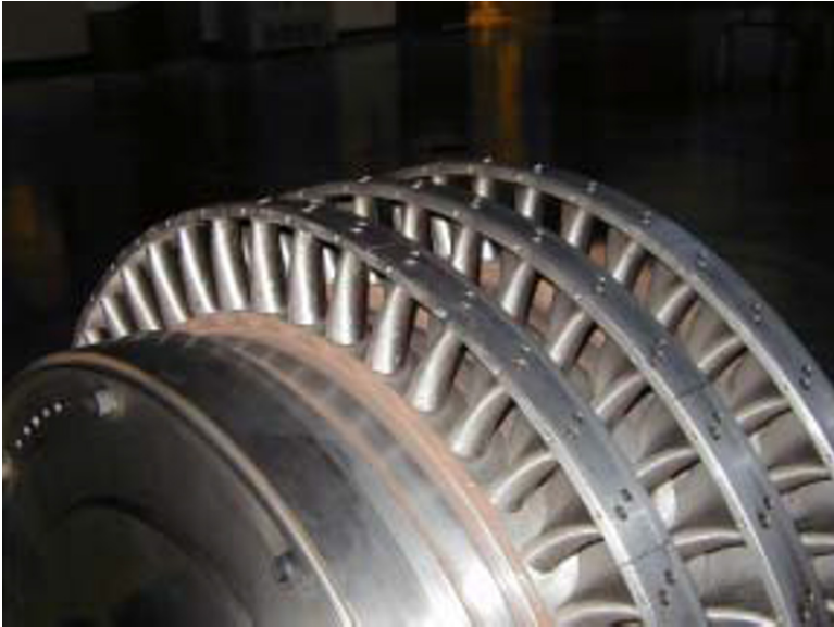
Fig. 1.4: A three-stage high pressure research turbine with bowed blades and tip shroud to reduce secondary flow and tip clearance losses
