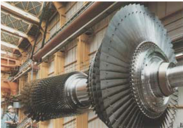
Fig. 1.9: Rotor unit of a heavy duty gas turbine with multi-stage compressor and turbine, compressor pressure ratio 15:1, (ABB-GT13E2)
