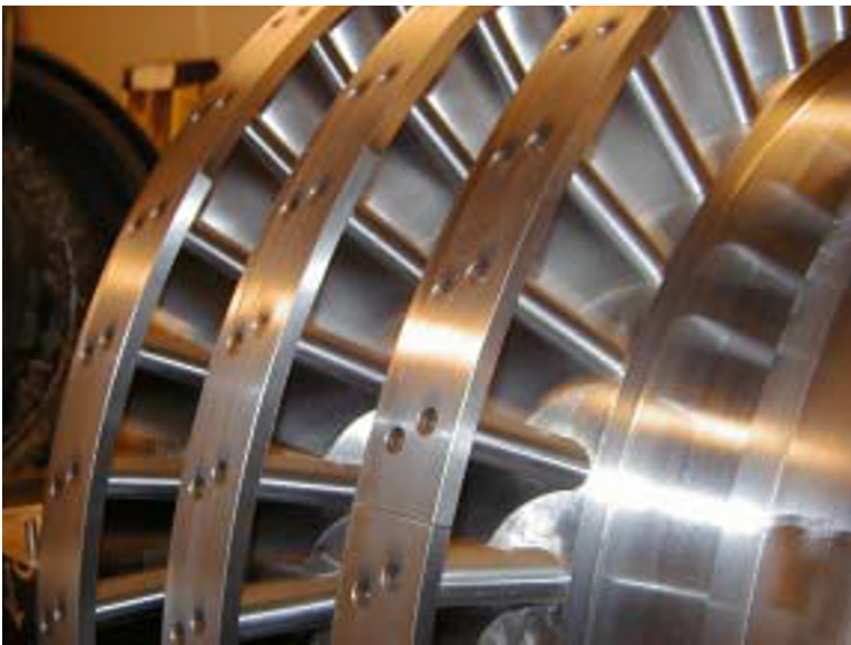
Fig. 1.2: A typical HP-steam turbine with the first control stage, inner and outer casings and labyrinth seal packets, (ABB Power Generation)
