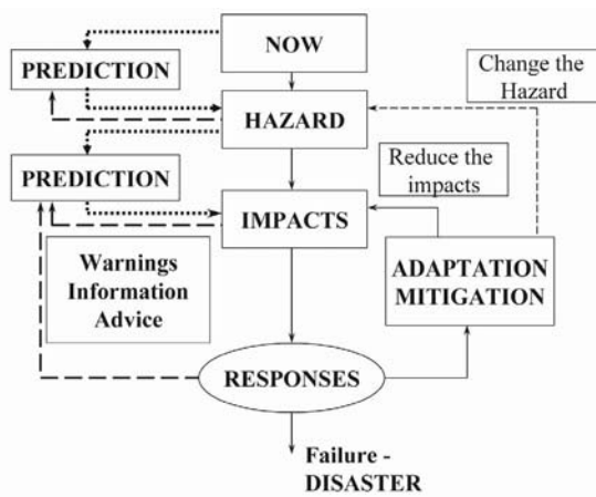
Figure 74.1: Role of prediction in providing warnings, information, and advice on the impacts and possible responses.
