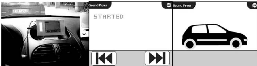
Figure 9-2. The Sound Pryer Prototype. A PDA and loudspeakers on the dashboard (left). The Sound Pryer Interface: Local play (middle) and remote play (right).
