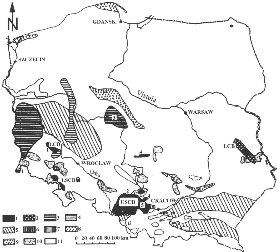
Fig. 1. Occurrence of principal mineral raw materials in Poland (Kozłowski 1983). Hard coal districts: 1, operating; 2, designed. Brown coal districts: 3, operating; 4, designed (1, Turossów, 3, Konin, 4, Beltchatów); 5, petroleum and gas districts. Metallic ore districts: 6, operating; 7, designed (1-copper, 2, 3, 4, 5, Pb-Zn); Chemical raw material districts: 8, operating; 9, designed (1-sulphur, 2, 3, rock-salt), Industrial stones: 10, operating; 11, designed.
