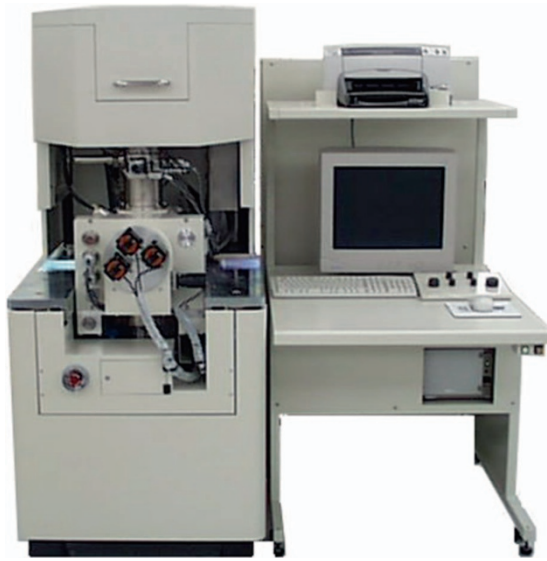
Figure 4-1. Schematic diagram of FIB equipment used for specimen preparation.
