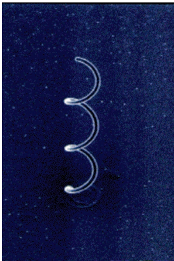
Figure 4-5. 3D fabrication of a spring coil.
