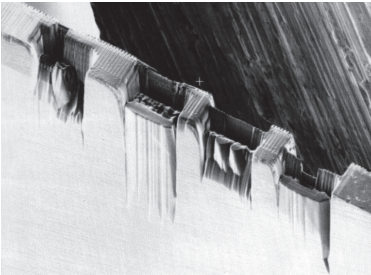
Figure 9.11. Planar semiconductor TEM specimen with four FIB TEM specimens cut at precise distances from the specimen top surface.
