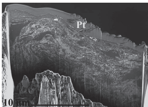
Figure 10.14. FIB image of a mechanically alloyed particle consisting of a mechanically alloyed mixture of Ti, Mg, and Ni. This single specific particle was placed on a TEM grid as shown in figure 14.
