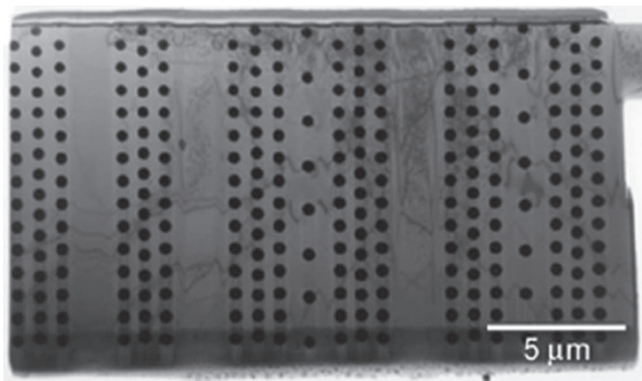
Figure 10.7. Low magnification TEM image showing plan view of over 200 W plugs prepared by EXLO.
