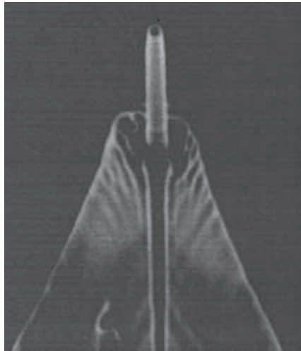
Figure 4-10. An 80 nm diameter tip FIB prepared for a scanning probe microscope.
