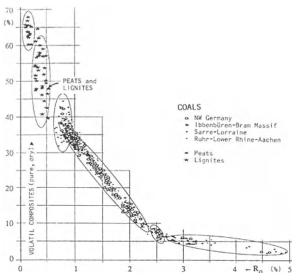
Fig. 6. Reinterpretation of the data of Teichmüller (1971). The correlation of the R_o reflectance with the volatile components on pure-dry material outlines several areas. From top to bottom, the areas of water expulsion and alcohol function, of decarboxylation, of expulsion of gaseous hydrocarbons, especially between 0.6 to 2.5 R_o and of expulsion of dry methane and probably of hydrogen, follow each other
