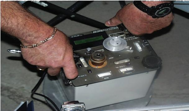
**FIG. 2. Onsite measurement using gravimeter equipment.**
