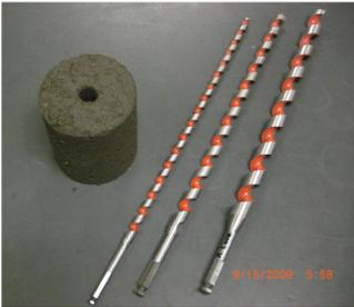
FIG. 4. Hole formation in soil specimen.
