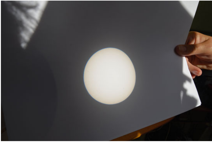
Fig. 7.3 Image of the sun projected onto a white piece of card (Courtesy of the author)
