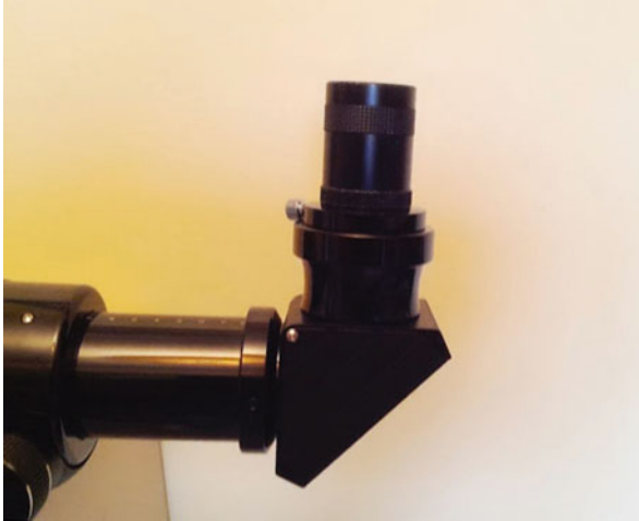
Fig. 4.6 Right angled Prism in use on a small telescope (Courtesy of the author)
