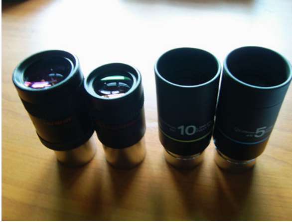
Fig. 4.4 A range of eyepieces for different objects. Long focal length=Wide field for deep-sky. Short focal length=Planets (Courtesy of the author)
