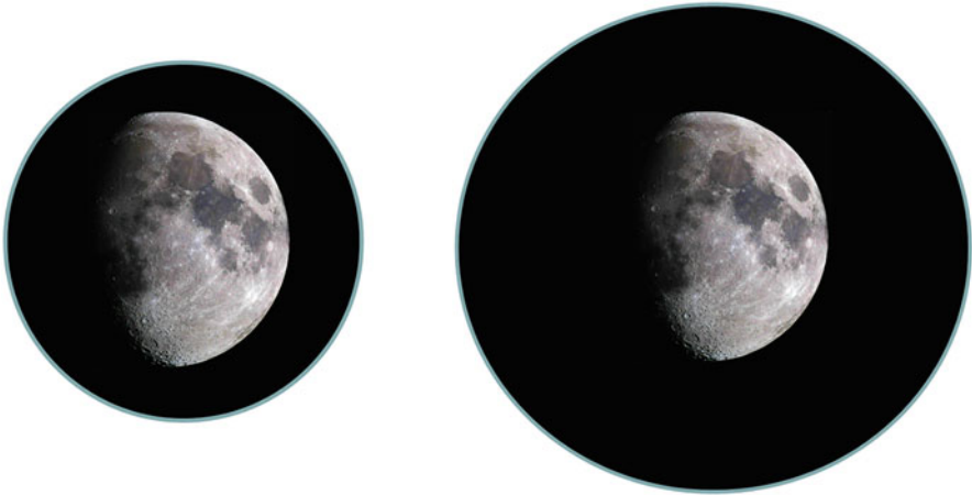
Fig. 4.3 Comparison of wide angle and normal eyepiece field of view (Courtesy of the author)
