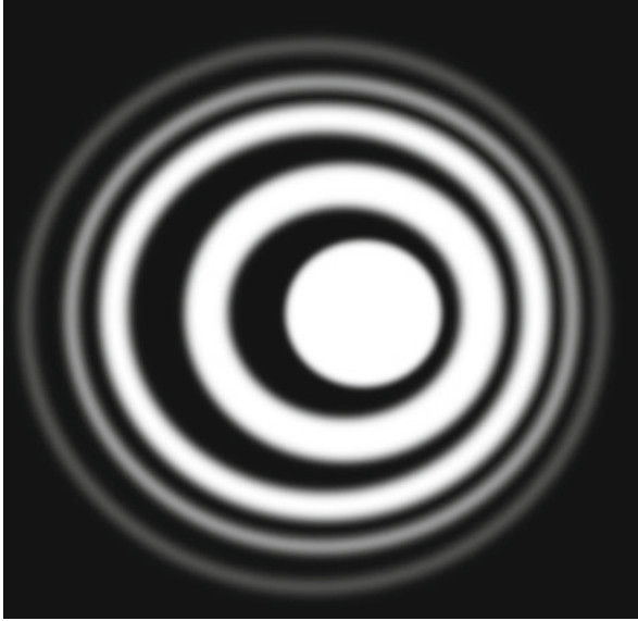
Fig. 6.5 Appearance of an airy disk in a badly collimated telescope (Courtesy of the author)
