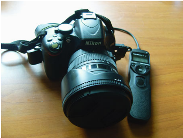
Fig. 13.1 The authors trusty DSLR and shutter release timer (intervalometer) for taking multiple images (Courtesy of the author)
