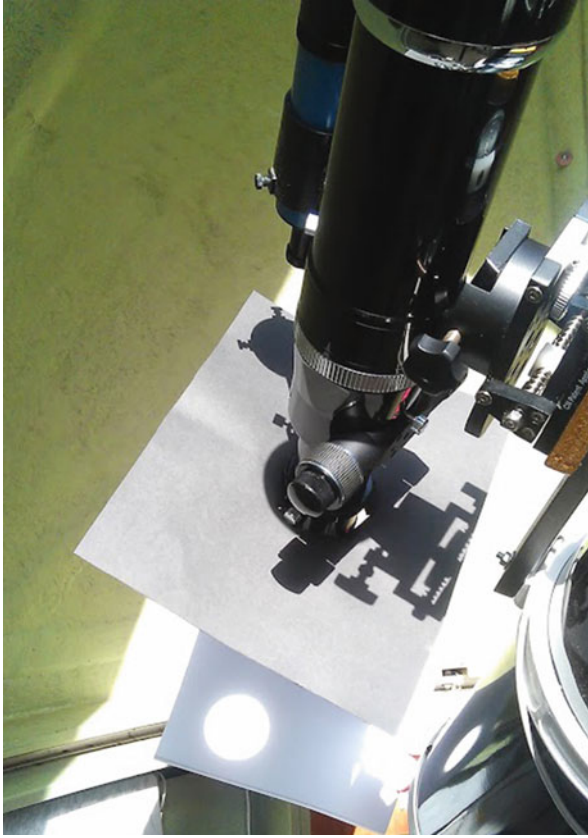
Fig. 7.2 Solar projection through a small telescope (Courtesy of the author)
