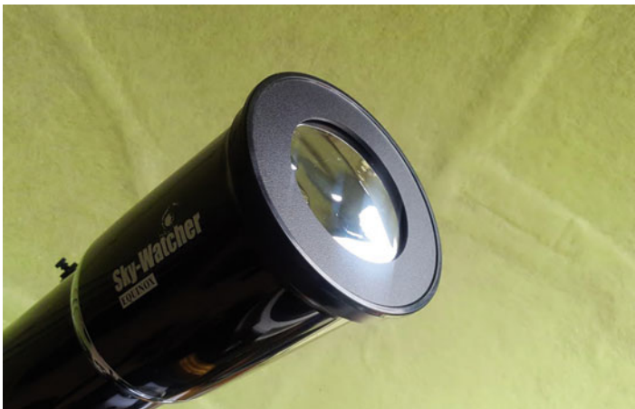
Fig. 7.5 A safe mylar filter securely attached to the end of a small refractor for direct viewing (Courtesy of the author)
