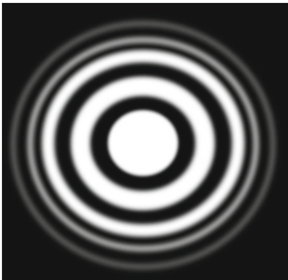
Fig. 6.4 Appearance of the airy disk in a telescope (Courtesy of the author)
