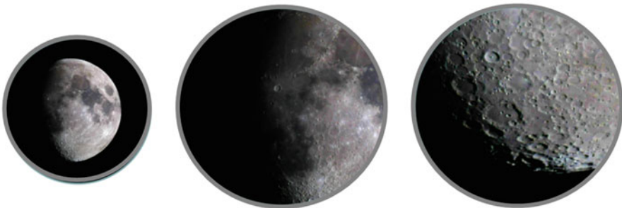
Fig. 4.2 Comparing eyepiece field of view at different magnifications (Courtesy of the author)
