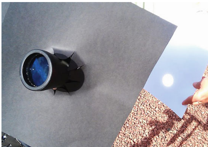
Fig. 7.1 Solar projection using binoculars (Courtesy of the author)
