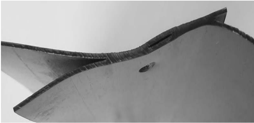
Figure 6.8 A typical dual hot wedge seam.
