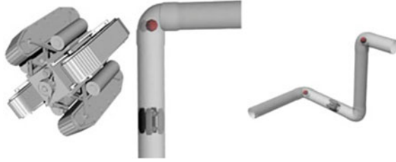
Fig. 2.8 Simulation environment. The 3-D model of the FAMPHER robot in the pipeline; red points denote guarding points
