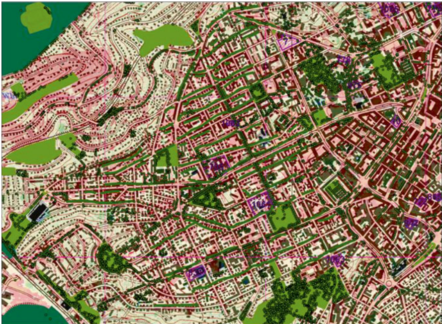
Fig. 10.14 Optimised design of street canyons in Stuttgart-West. Green lines marking street canyons, where the thermal stress is reduced due to facade greening of the use of cool materials for facades. Green circles marking possible positions for trees
