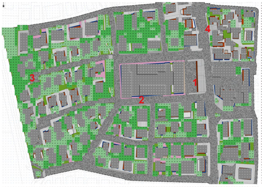
Fig. 7.4 The model area in ENVImet used for the simulations of the “AsIs”, “Cool pavements” and “Cool roofs” scenarios. The red numbers identify four characteristic points for which air temperature at 2 m above ground has been considered in the study
