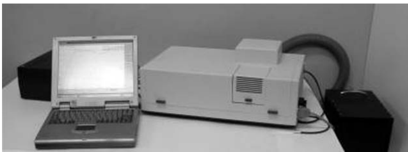
Figure 19. Bioanalytical system consisting of the portable CD-spectrometer combined with the biosensing unit based on the liquid-crystalline DNA dispersions.
