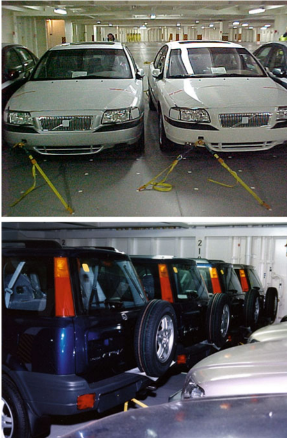
Fig. 19.1 Lashed cars secured on ship decks
