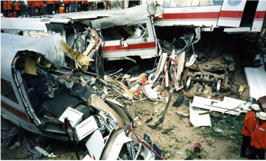
Fig. 1.9 The destruction of rear passenger cars that were pushed into each other and crashed into a road bridge (Eschede accident, 3rd of June, 1998, photo by Nils Fretwurst)
