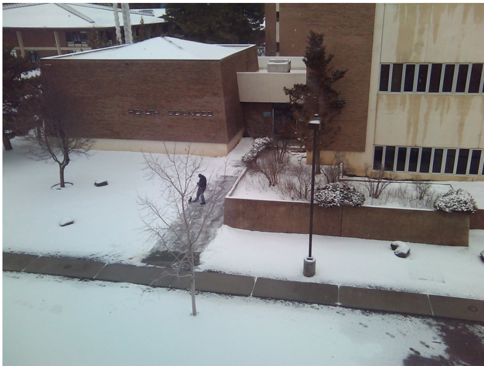
Figure 8. Comparison between heating and non-heating sidewalks on the east wing of Engineering Building taken at 10am (01/28/2013).
