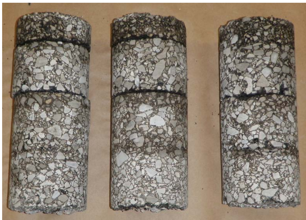
Figure 3. Cores showing layer debonding.
