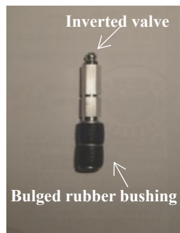
Figure 3. Installation of grouting needles.
