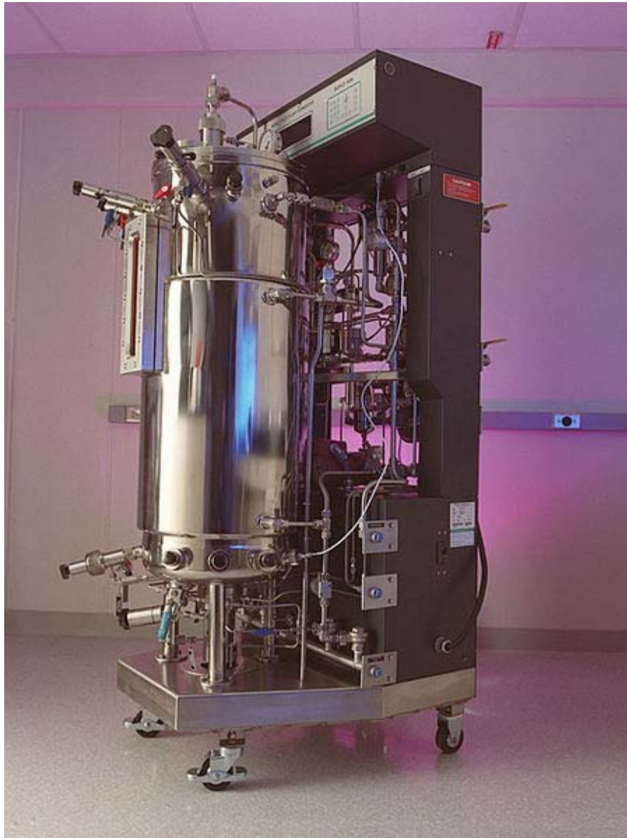
A closed bioreactor used in cellulosic ethanol research
