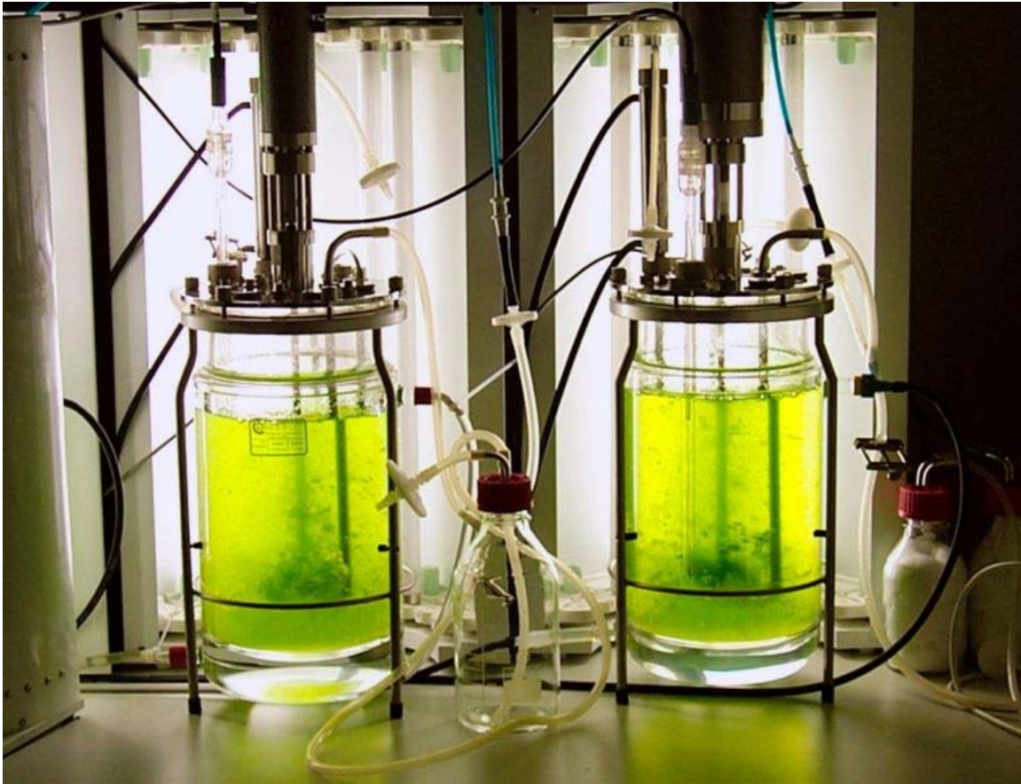
Moss photobioreactor with Physcomitrella patens
