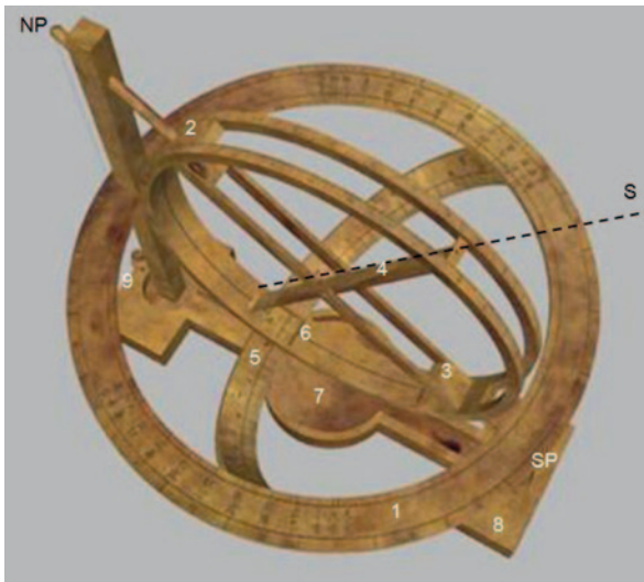
Fig. 11 South-determining Sundial (reconstruction drawing). 1: Fixed Horizontal ring is graduated to indicate the 24 azimuth directions as well as the azimuths of sunrise and sunset during the 24 Fort-nightly Periods. It was held up by the top of the 0.59 c (12.2 cm) high south column (hidden) and used for equalizing sunrise and sunset at the summer solstice; 2: Four Displacements ring which received its pivots in the 0.11 c (2.2 cm) below the top of 1.1 c (22.7 cm) long north column and 0.038 c (0.7 cm) below the top of the south column. And it was graduated with the degrees of the celestial circumference, from North 16 d to 167 d there was a slot in the ring and engraved a meridian line on the inside of the rest; 3: Cross-struts carrying a sighting-alidade; 4: Alidade having a round hole one side and a square aperture the other side; 5: Equatorial half-ring inscribed day time 'marks'; 6: Square aperture for reading the 'marks' of the equatorial half-ring; 7: Round pool 0.26 c (5.3 cm) in diameter having water-grooves reaching to the both ends and encircling the columns; 8: Stand 1.25 c (25.8 cm) long, 0.4 c (8.2 cm) wide at both ends for a distance of 0.2 c (4.1 cm), and 0.1 c (2.0 cm) wide and 0.85 c (17.5 cm) long waist; 9: Weight for leveling opposite to the cross below. NP: celestial North Pole; SP: South Pole; S: Solar rays. (Adapted from Nam 2002, p. 71)
