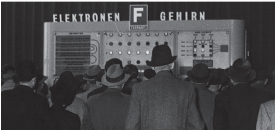
Fig. 6 The Nimrod at the Berlin Industrial Show on 6 October 1951. It is a 9 by 12 by 5 feet machine that contains 480 vacuum tubes and executes its program almost independently. ( http://www.heise.de/newsticker/meldung/Vor-50-Jahren-fing-alles-an-das-erste-Elektronenhirn-in-Deutschland-51722.html )
