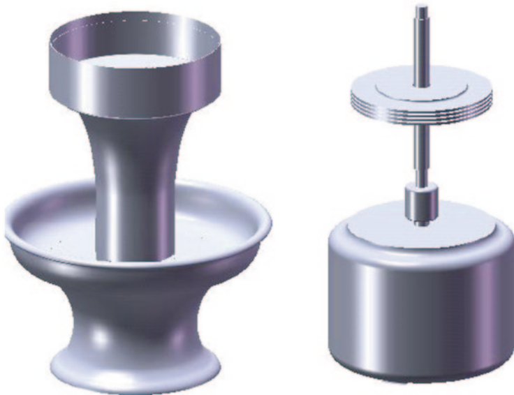
Fig. 8 The third variant of Tesla’s table fountain and its propelling system with an electric motor (CAD models)
