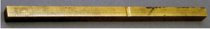
Fig. 6 The Standard Measure. Reconstructed in 1740 under Yeongjo from the relics made in Sejong's reign in 1437. It was made of bronze, 24.6 cm long, 1.2 cm wide and 1.5 cm high rectangular and used until the end of nineteenth century. It is composed of the graduations in half-scale and uses of five standard measures on four-sides, two measures on the front surface; Ju-cheok 10.35 cm for making the astronomical instruments and Yegi-cheok 13.7 cm for making ceremonial vessels; Pobaik-cheok 24.6 cm for clothing and trading on the second side; Yeongjo-cheok 15.4 cm for the constructions on the third side; Hwangjong-cheok 17.3 cm for making musical instruments on the fourth side. Doubling the length of each ruler make up one cheok . The graduation of a foot cheok divided into ten chon , and a chon into ten inch bun following the decimal system. Collection of the National Palace Museum of Korea, Seoul. (Photo courtesy of Nam MH)
