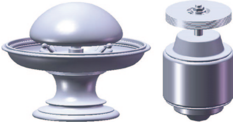
Fig. 18 Full view and the propelling system of the fourth variant of Tesla's table fountain (CAD models)
