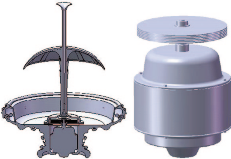
Fig. 14 Vertical section and the propelling system of the second variant of Tesla's table fountain (CAD models)
