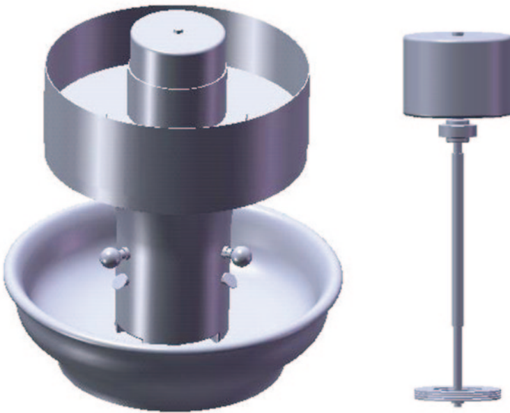
Fig. 4 The first variant of Tesla's table fountain and its propelling system with an electric motor (CAD models)
