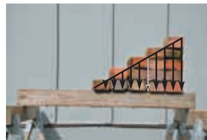
The pile of brick creates an approximate triangular distributed loading on the board. (© Russell C. Hibbeler)
