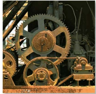
The gears used in the operation of a crane all rotate about fixed axes. Engineers must be able to relate their angular motions in order to properly design this gear system. (© R.C. Hibbeler)
