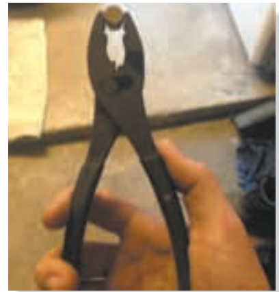
Common tools such as these pliers act as simple machines. Here the applied force on the handles creates a much larger force at the jaws. (© Russell C. Hibbeler)
