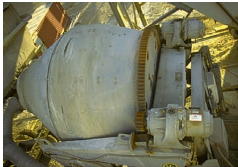
The work of the torque or moment developed by the driving gears on the motors is transformed into kinetic energy of rotation of the drum. (© R.C. Hibbeler)
