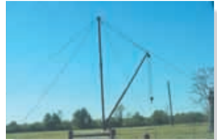
This crane is a typical example of a framework. (© Russell C. Hibbeler)
