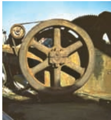
This flywheel, which operates a metal cutter, has a large moment of inertia about its center. Once it begins rotating it is difficult to stop it and therefore a uniform motion can be effectively transferred to the cutting blade. (© Russell C. Hibbeler)
