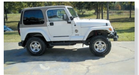
The jeep leans backward due to its inertia, which resists its forward acceleration. (© R.C. Hibbeler)
