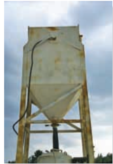
The walls of the tank must be designed to support the pressure loading of the liquid that is contained within it. (© Russell C. Hibbeler)
