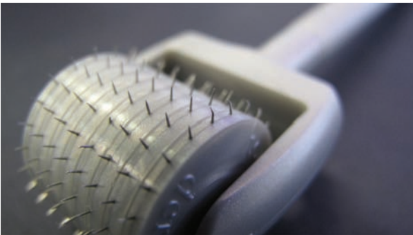
Figure 9.17 Professional device's micro-needles after acne scars' treatment: note how tips are bent like a fishhook.
