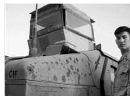
fig. 19 | A High Mobility Multipurpose Wheeled Vehicle (HMMWV) modified with Popemobile glass
