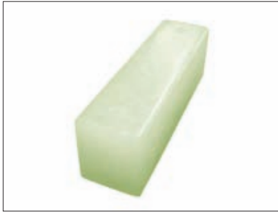
fig. 3 | Brick made of recycled optical borosilicate glass
