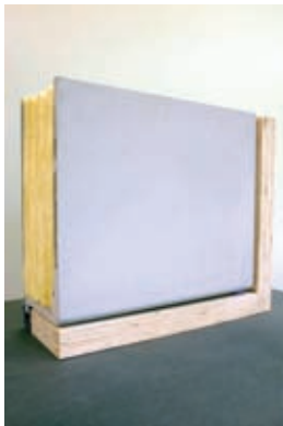
fig. 8 | Fiber-reinforced concrete for heat conduction and stability
