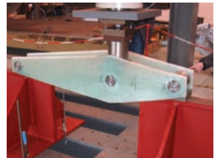
fig. 7 | Failure at approximately 300kN
