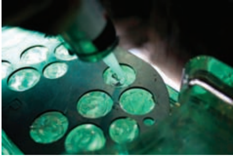
Blocks being joined with transparent adhesive
