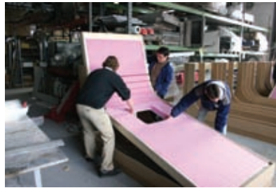
fig. 9 | A panel of GRP skin, PU foam, and fiber-reinforced concrete for the production of multifunctional system components
