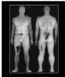
figs. 16 + 17 | Passive Millimeter Imaging (PMI), used to detect hidden weapons or contraband in clothing, bags, and vehicles
