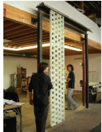
fig. 7 | Testing configuration, mock-up of borosilicate brick curtain
