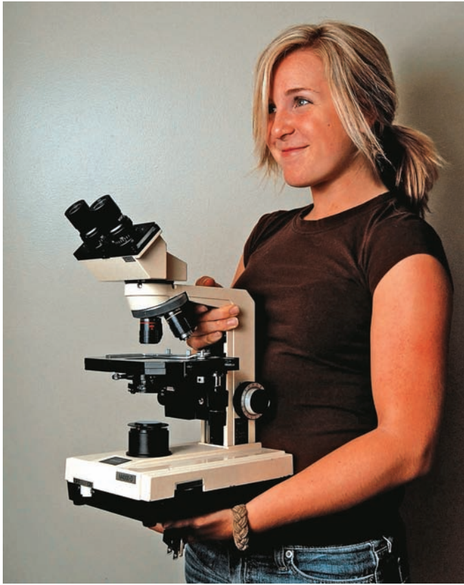
Figure 3.1 Proper Technique for Carrying a Microscope.
