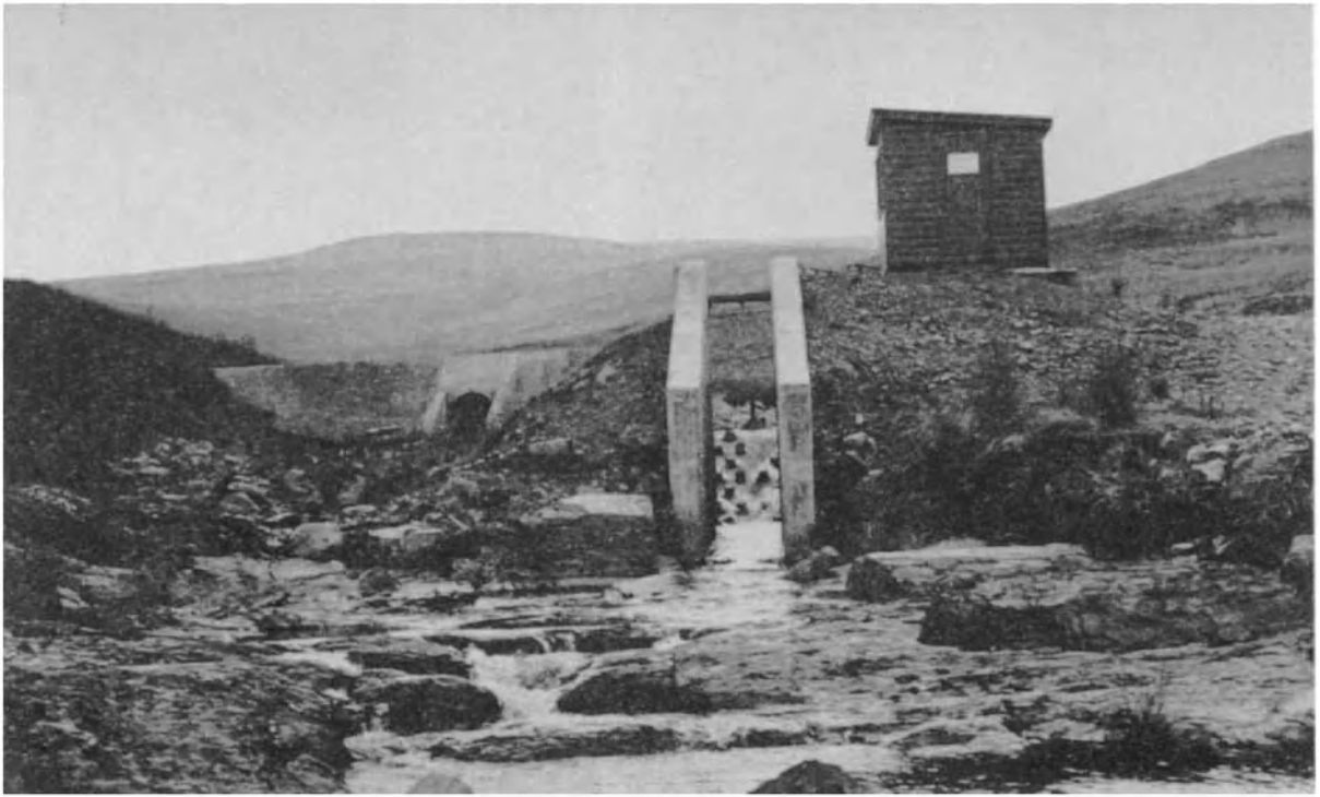
Figure 5.1 The dry weather flow of the River Wye, Plynlimon. At times of high flow the water can fill and overtop the measurement flume.
