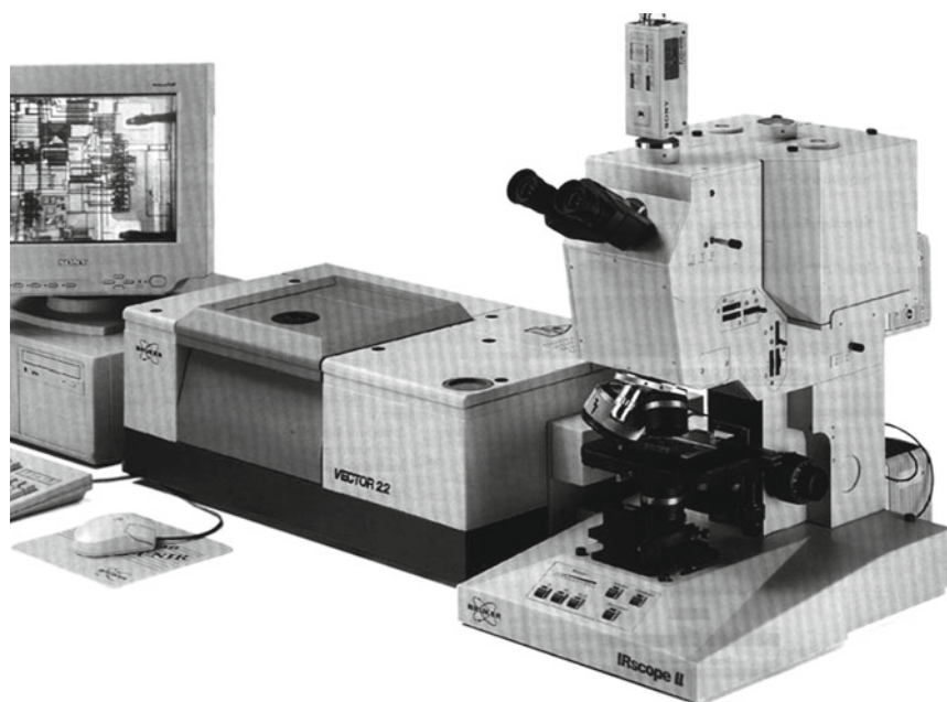
Fig. 10.1 A representative photo of the FTIR microscopy instrument used in this study
