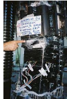
Figure 14: Failure of the CFRP layers of the mid-part.
