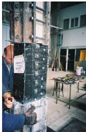
Figure 4: Confining steel brackets and partial CFRP confinement at the mid-part.
