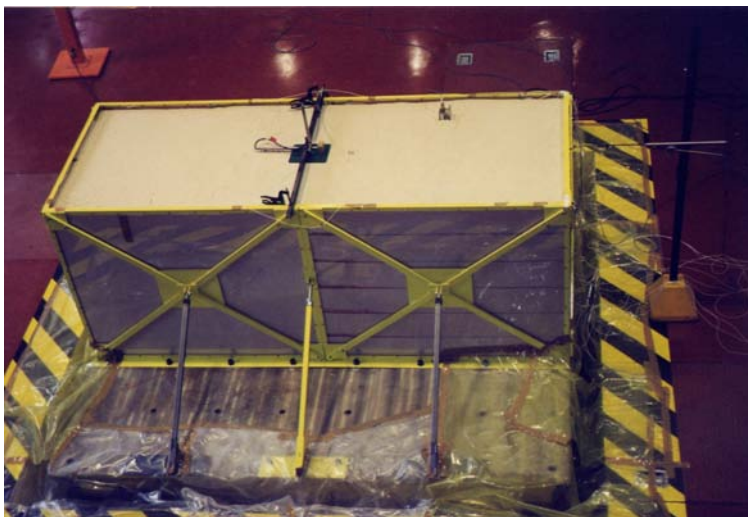
Figure 1: Photograph of the box, filled with sand, on the shaking table.
