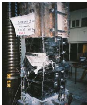
Figure 10: Tensile failure of CFRP layers. Considerable effectiveness of partial confinement.
