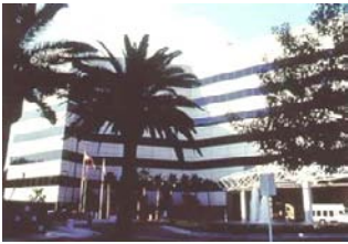
Figure 10: The University of Southern California Hospital at Los Angeles protected by LRBs and completed in 1991, that withstood the 1994 Northridge earthquake without any damage, contrary to other conventionally founded hospitals located in the neighbourhood (e.g. the Olive Hospital, which had just been repaired after suffering severe damage during the San Fernando earthquake).
