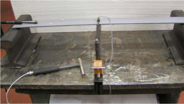
Figure 3: Model of bridge with dampers.
