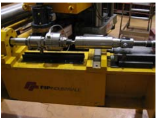
Figure 23: Left and centre: seismic improvement in progress for the Dome of Siena, by means of recentring viscous dampers (VDs), to avoid the overturning of the façade. Right: view of a VD during tests.
