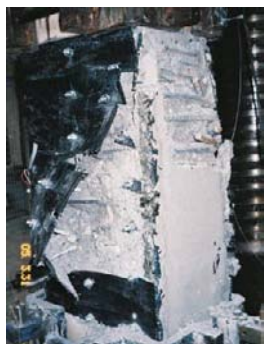
Figure 9: Failure of anchor bolts. Low effectiveness of partial confinement.
