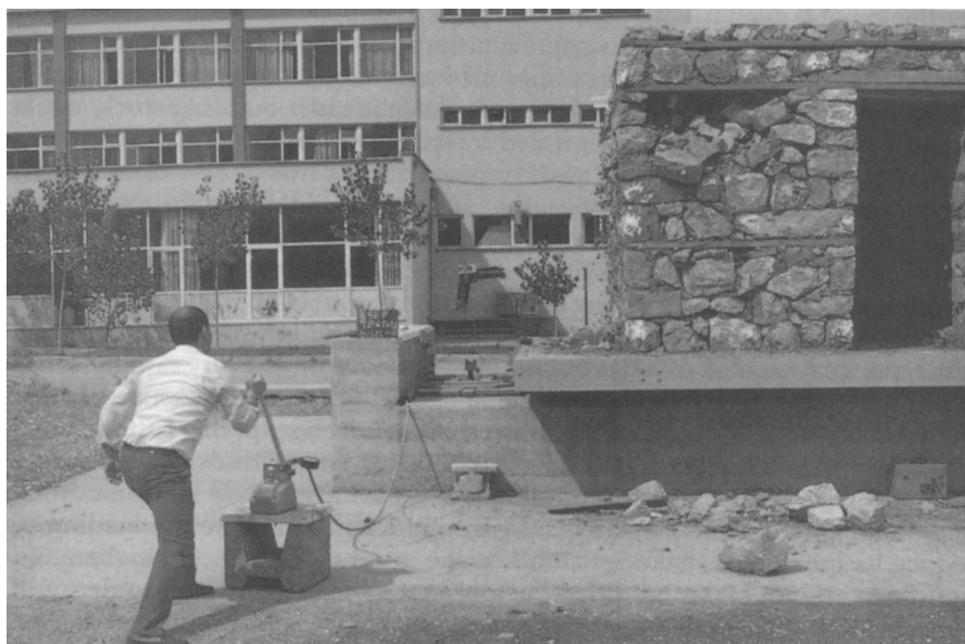
Figure 8.11 The effectiveness of earthquake-resistant construction can be demonstrated using destructive experiments on full-sized buildings. Here a full-size rural masonry building is shaken apart on a simple 'impulse table' where a concrete slab vibrates on rubber bearings
