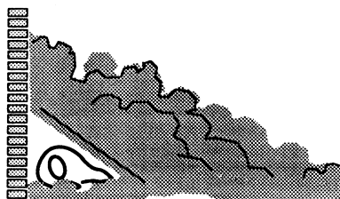
Standing walls may indicate the possibility of a void at their base
