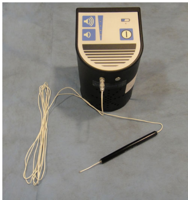
Fig. 3.1 VTI surgical Doppler 9.3 MHz and a disposable probe flow detector (Vascular Technology Int., USA)
