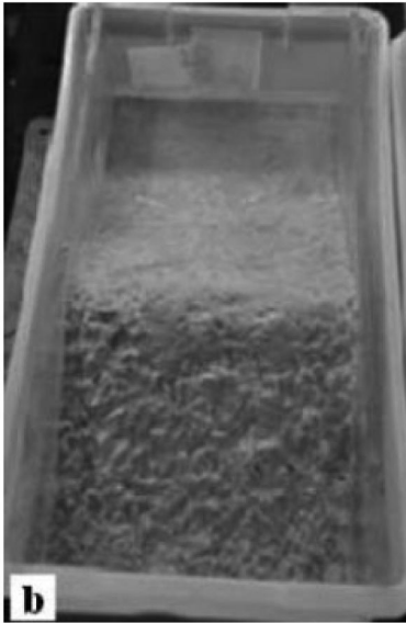
Figure 11. A levee model after treatment using biogrout.
