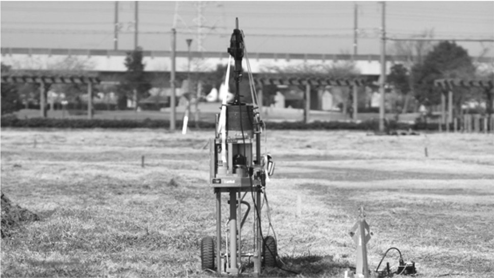
Figure 2. View of “Dynamic Weight Sounding (DWS)” test.
