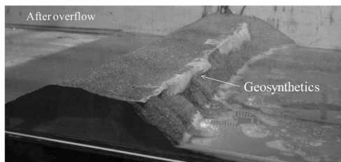
Photo 8. Reinforced earth bank after overflow in Case-4.
