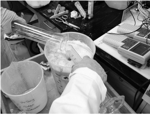
Figure 15. Production of biogrout using solutions made of limestone fines and corn cobs with the addition of biomass and urea.
