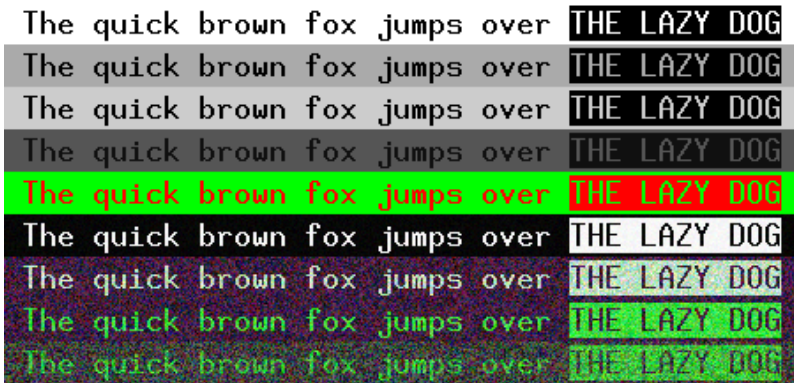
Fig. 7. Test image for text contrast in compromising emanations from DVI cables
