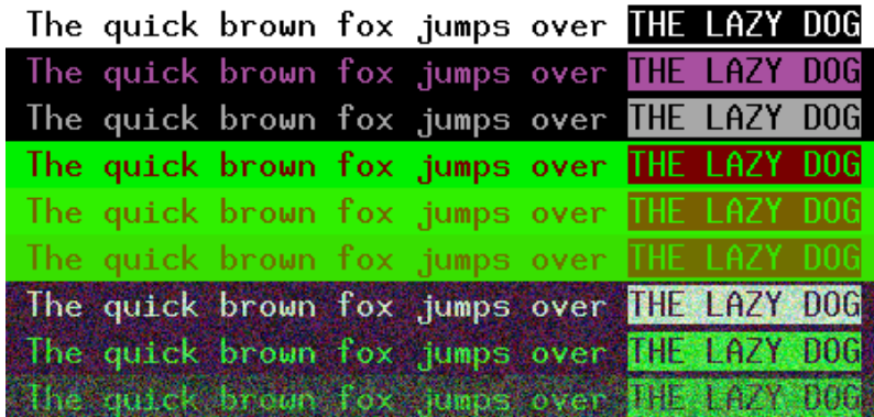
Fig. 5. Test text to compare the emission characteristics of selected foreground and background color combinations
