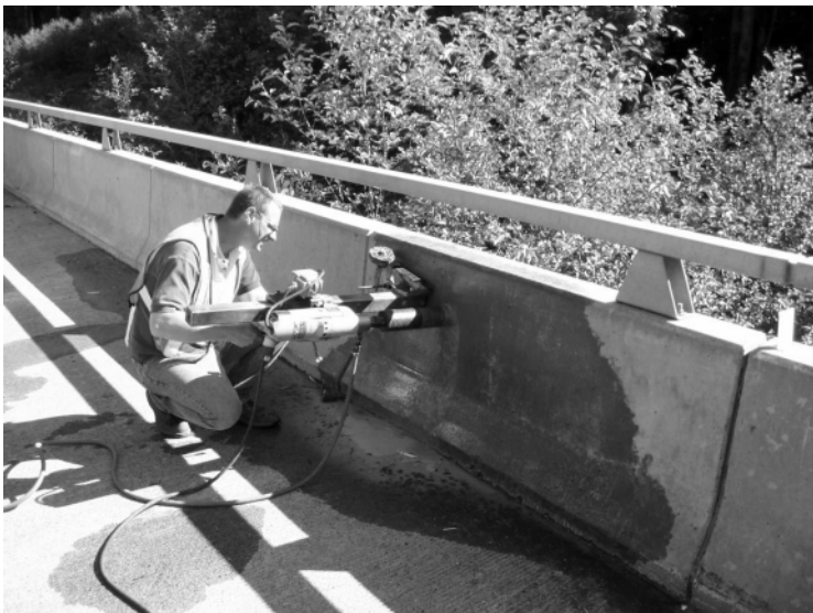
14.24 Waterloo Creek Bridge – core sample extraction.
