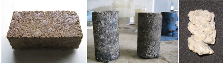
Fig. 23.7 Use of plastic to make instant strong construction materials on site
