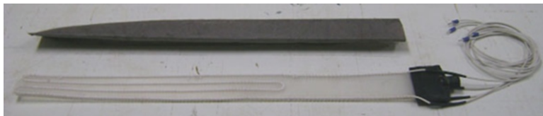
Fig. 19.5 Flexible heater wire combined with PVD
