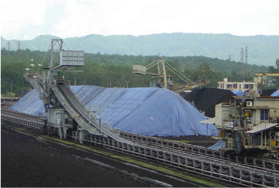
Fig. 13.1 Storage of lignite piled up by belt-conveyor at the Mae Moh mine under operation of the Electricity Generating Authority of Thailand
