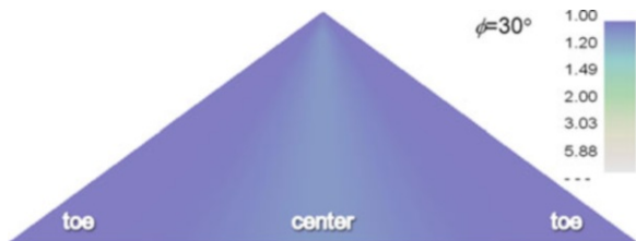
Fig. 13.11 Distribution of the safety factor in a two-dimensional heap body with \phi = 30^\circ
