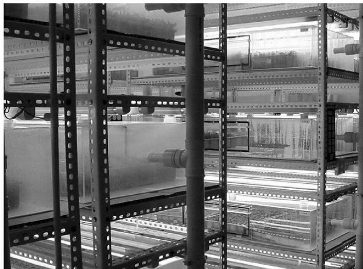
Figure 2. A photoautotrophic micropropagation system using large vessels with forced ventilation, installed for commercialization in Kunming, Yunnann Province, China.
