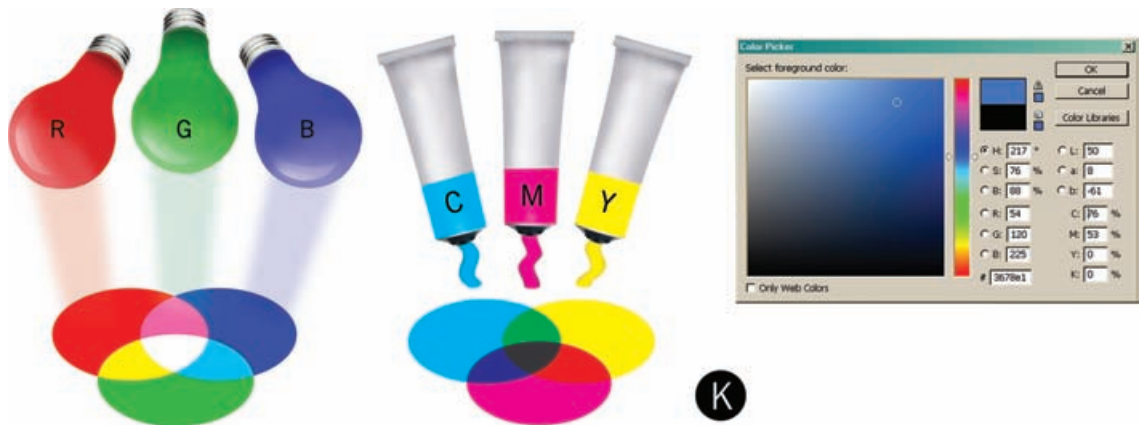
FIGURE 3-7 The RGB color model is based on light. The CMYK color model is based on ink (pigments). The color picker in Adobe Photoshop permits the use of RGB, CMYK, Web-safe, and Pantone color models.
