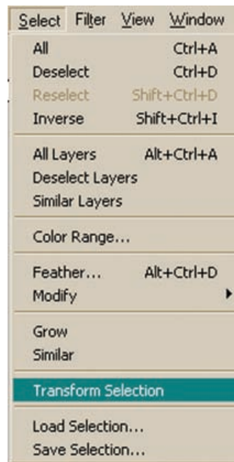
FIGURE 5-9 Scale and reposition the selection area without affecting the pixels inside by using the TRANSFORM SELECTION command.
