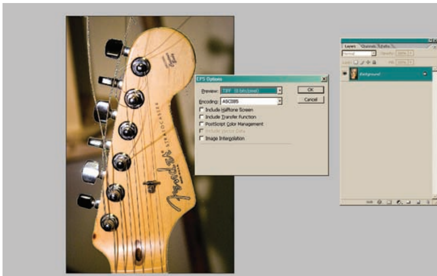
FIGURE 5-38 When setting EPS OPTIONS, use ASCII85 for Windows and Binary Encoding for Macintosh. Always use TIFF 8 bit preview. Make sure other boxes are unchecked.
