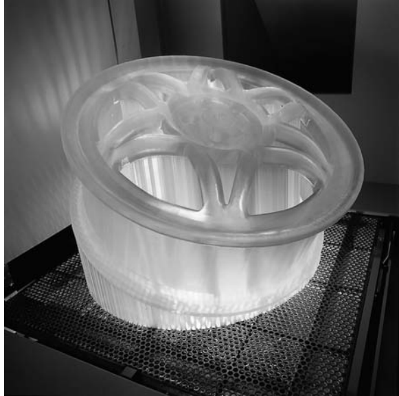
FIGURE 33.3 A part produced by stereolithography. (Photo courtesy of 3D Systems, Inc.)
