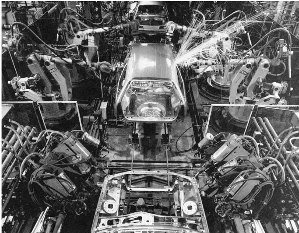
FIGURE 38.16 A portion of an automobile assembly line in which robots perform spot-welding operations. (Photo courtesy of Ford Motor Company, Dearborn, Michigan.)
