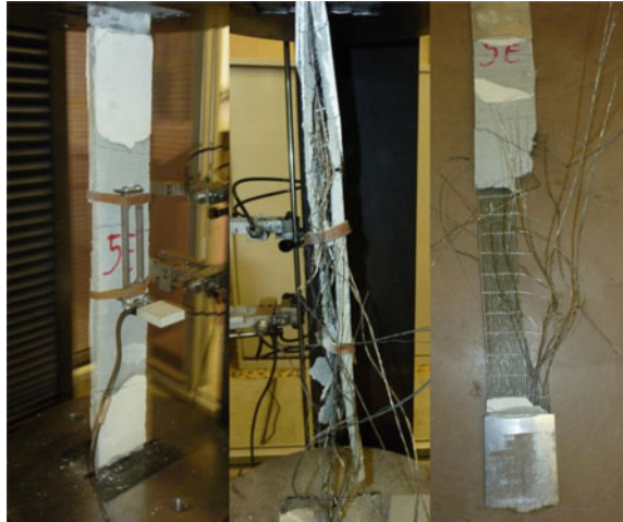
Fig. 9.8 Cracking, splitting and failure of the steel FRCM specimens
