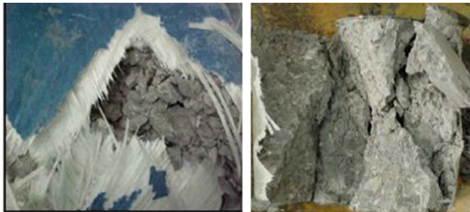
Fig. 5.11 Comparison of highly and lightly confined concrete appearance after jacket rupture
