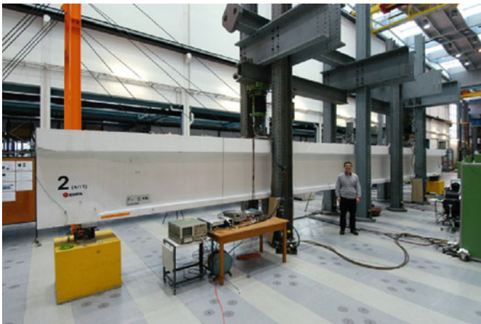
Fig. 7.11 Large-scale prestressed concrete bridge girder testing at Empa (Czaderski and Motavalli 2007)
