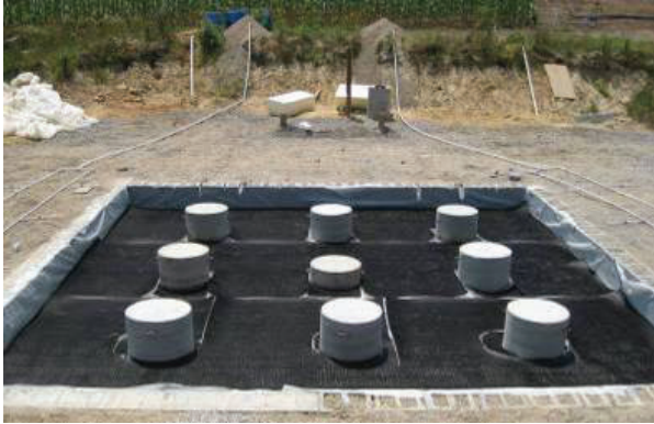
FIG. 7. CSE test facility with 9-column array.
