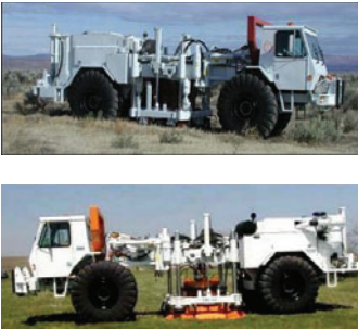
FIG. 19. In-situ dynamic measurements: (a) the Liquidator; (b) T-rex vibrator; (c) comparison of G/G_{max} reduction curves from field and lab testing on sands (Stokoe et al. 2008).
