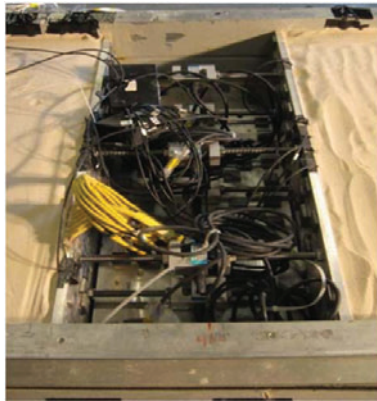
FIG. 11. Photograph of the cross-braced, U-shaped structure model with sand backfill. Note the load cell on each strut.
