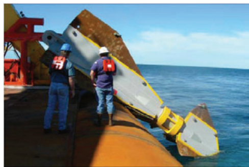
(b) Deploying OmniMax anchor
