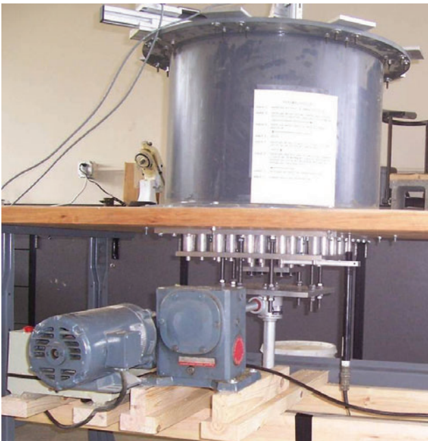
FIG. 2. Bench-scale test apparatus showing soil tank above the bench and 5 by 5 array of columns below the bench.
