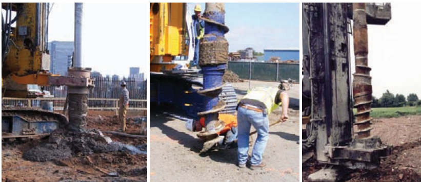
FIG. 9. Drilled Displacement Tools.
