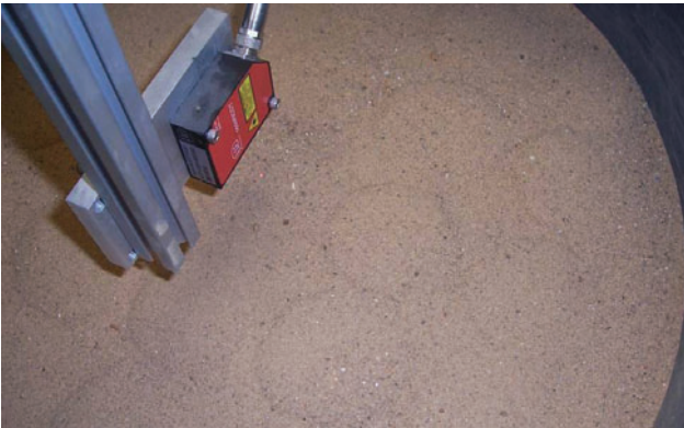
FIG. 4. View inside soil tank of bench-scale test apparatus showing differential settlement of sand above columns.
